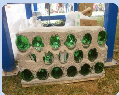
Sample wall made from bottles by SIT students
